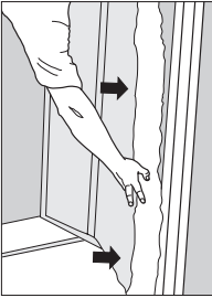
THERMAFIBER Sound Attenuation Fire Blankets fit snugly between steel studs
